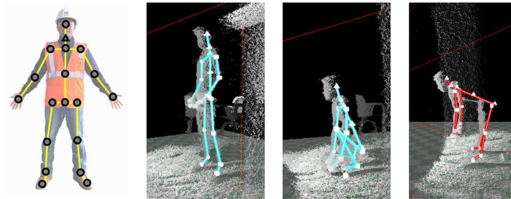
*Figure 3:* (left to right) Major joints in human skeleton, joints captured by Kinect camera for (i) standing, (ii) good lifting and (iii) bad lifting positions
