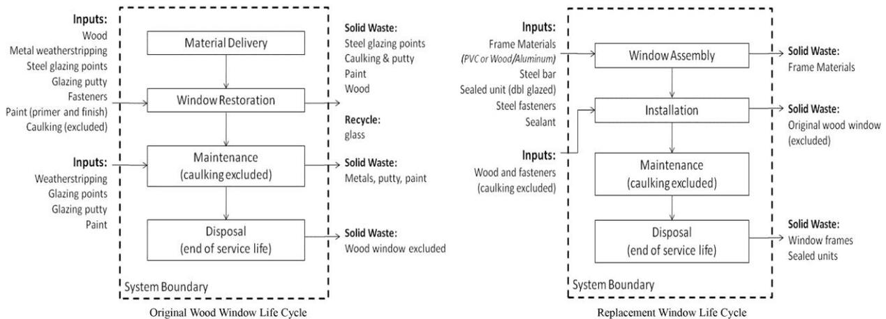
Figure 1: Original and replacement window life cycle.
