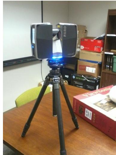
Figure 2b: 3D Laser Scanner
