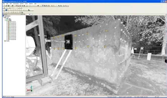
Figure 4b: 3D scan view of west wall during Out-of-plane loading
