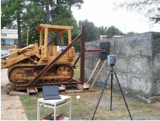
Figure 4a: Out-of-plane loading on west wall
